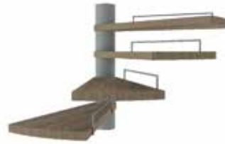
Steel riser bars
