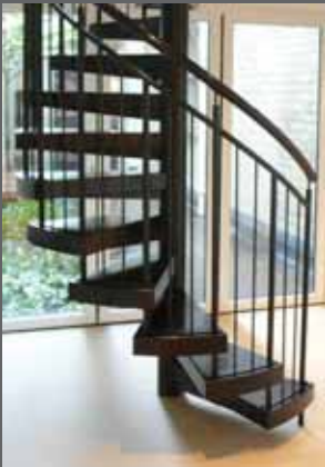
Bottom right: Spiral with walnut treads, external stringer and stainless balustrade.
