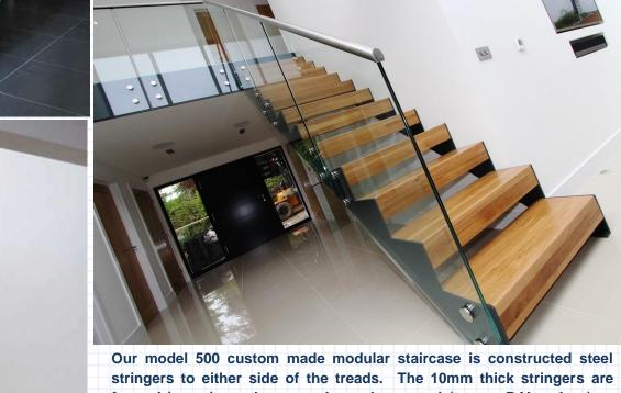
formed in various shapes and powder coated (to any RAL colour) or supplied in stainless steel.
